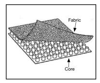
The Drain Max 500 Series is designed for use with the Drain Max water-proofing systems in vertical installations requiring high compressive strength and flow capacity. Use is suitable in selected horizontal applications.
