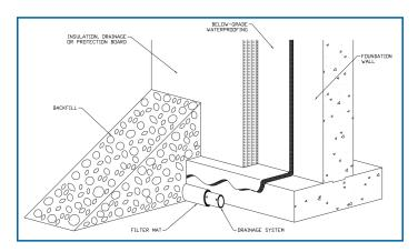
Drain tile or strip drain must be installed as per the manufacturer's instructions to ensure proper removal of water from the foundation walls and footings. Backfill must be graded to direct surface water away from the exterior foundation walls.
